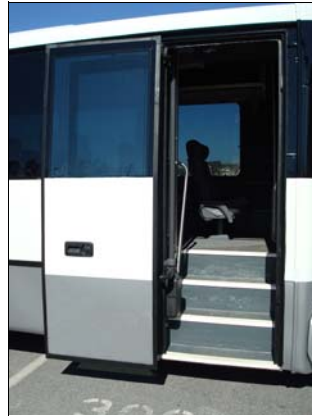
Bode air-operated entrance door offers a wide entrance area with a weather-proof, wind-resistant fit.
